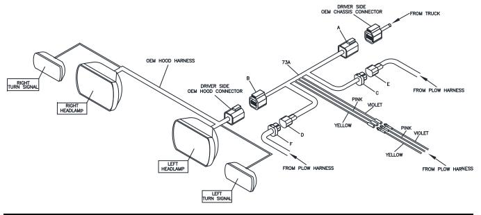
Figure 1. Ford F-650 & F-750 Headlight Adapter Installation
