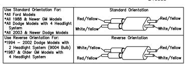
Figure 2. Vehicle Option Connector
